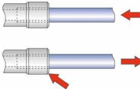
**Mounting:** Insert tube as far as it will go into the connection
